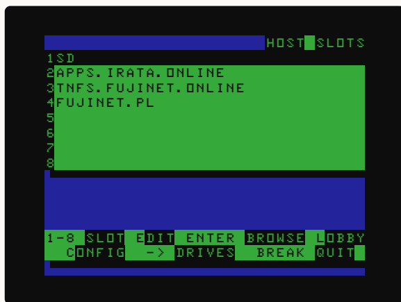
Figure 10. The Host Slots screen. Slot 1 is the microSD card; the others hold network libraries.
