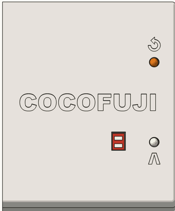
Figure 2. Cartridge top: lamps, model switches, and markings.
