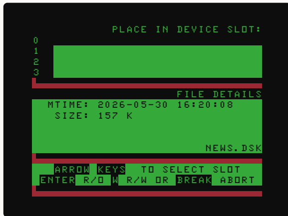
Figure 13. Choosing a drive slot. Drive 0 is the one your Computer boots from.
