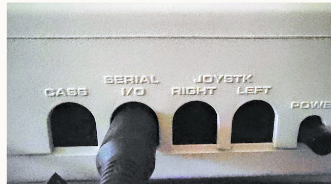
Figure 4. The serial plug in the SERIAL I/O jack — mind the look-alike CASS jack next door.
