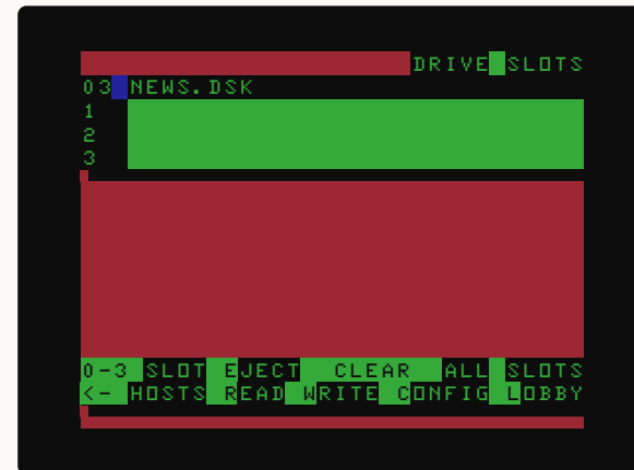
Figure 14. Drive Slots. Reading a line: drive number, the host it came from, a colored mode block, and the image's name.
