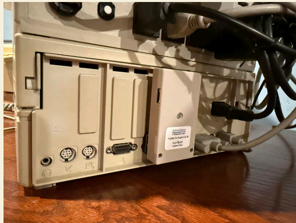
Figure 2-3. FujiNet on the IIGS
